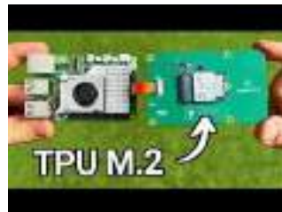
RPI series Possibly with HAT for accelerating machine learning (TPU: Tensor Flow Unit)
