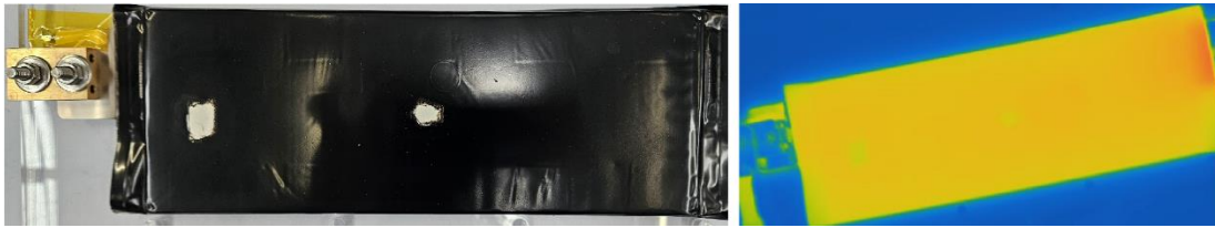
Figure 6 Coating the cell with matte black paint, an area was masked and then uncovered, leaving a reflective patch. Left) the painted cell, Right) the thermal image.
