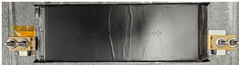
Figure 3 Cell sprayed with matt black paint (Ambersil).
